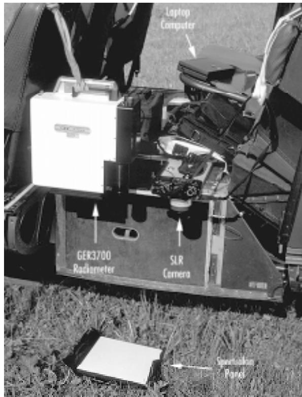
Figure 3. Helicopter Instrument Setup And Calibration Panel
