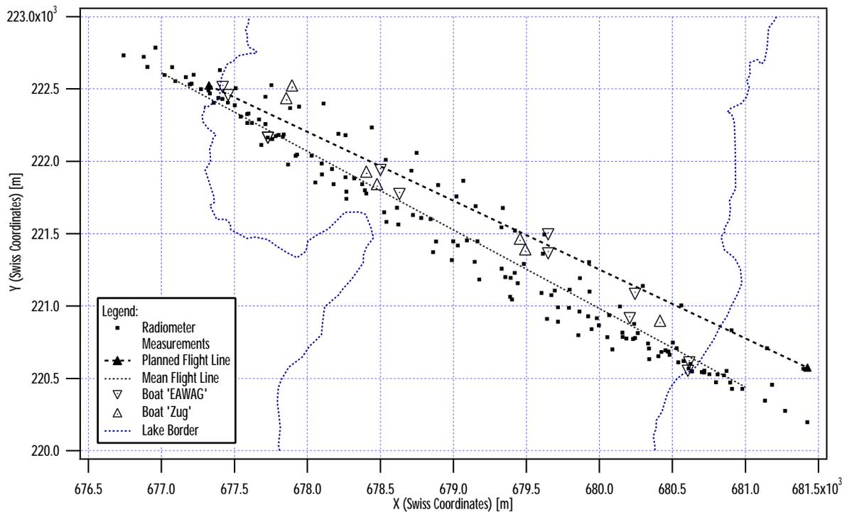
Figure 2. Measurement Point Distribution Of The Transect Flown
