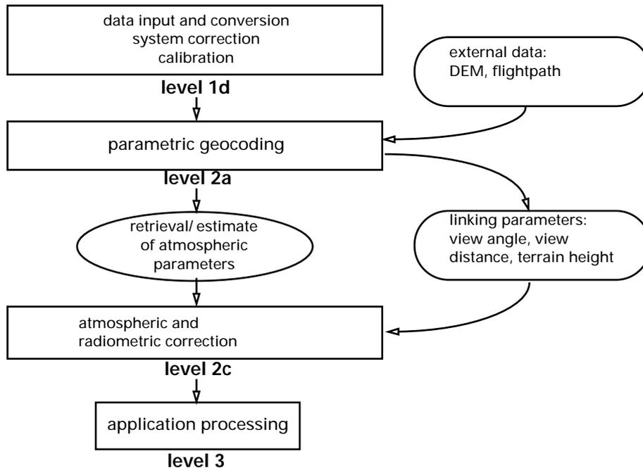
**FIGURE 1: A complete processing chain including parametric geocoding algorithm and terrain dependent atmospheric correction.**
