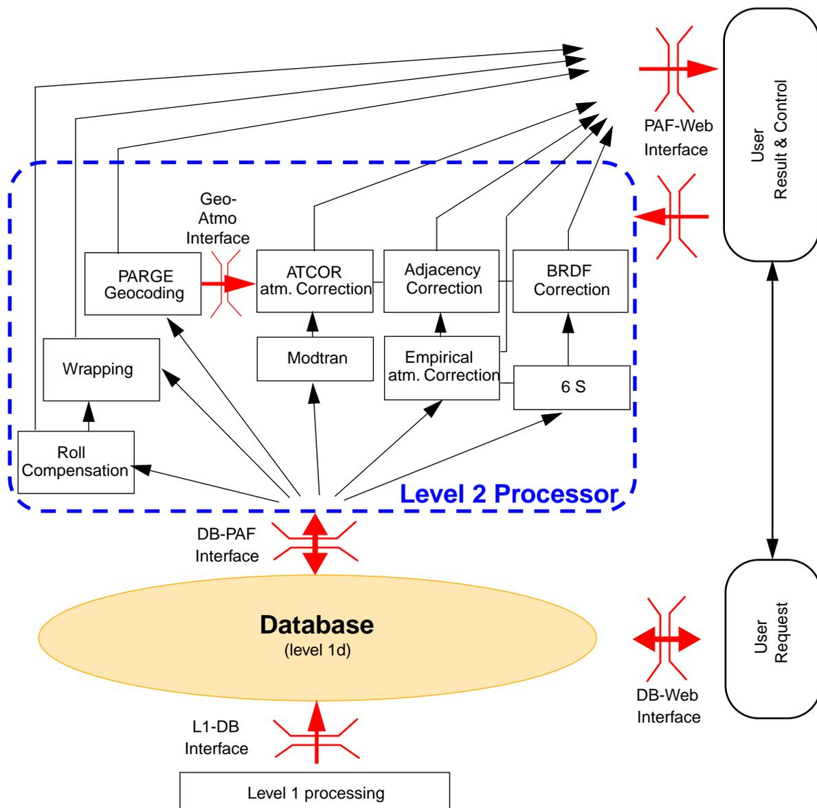
**FIGURE 2: The interface design between the single modules for the APEX level 2 processor.**
