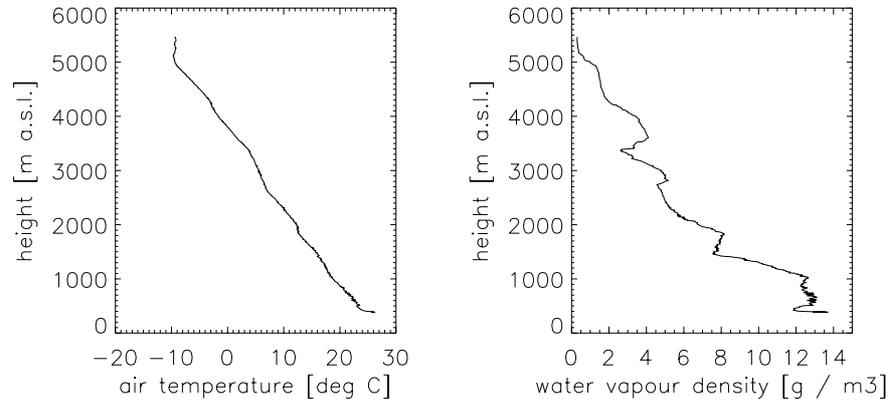
Figure 5 Typical temperature and water vapor density profile on a clear summer morning.
