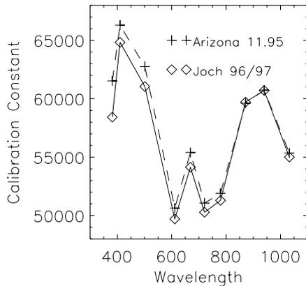
Figure 3 Calibration constants determined at Mount Lemmon (1995), at Jungfrauoch (1996), and Weissfluhjoch (1998); derived by the modified Langley plot method.
