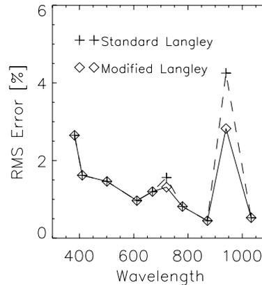
Figure 4 RMS deviation of 6 calibration runs between fall 1995 and winter 1998 for the standard and the modified Langley plot.
