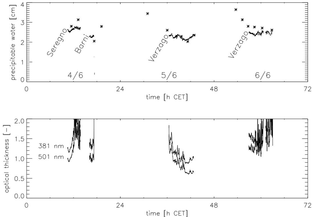
Figure 8 Top: precipitable water measured by radio sondes (asterisks) and by the solar radiometer (solid line) at Seregno, Barni and Verzago. June 4 - 6, 1998. Bottom: optical thickness of the radiometer channels 1 (381 nm) and 3 (501 nm).
