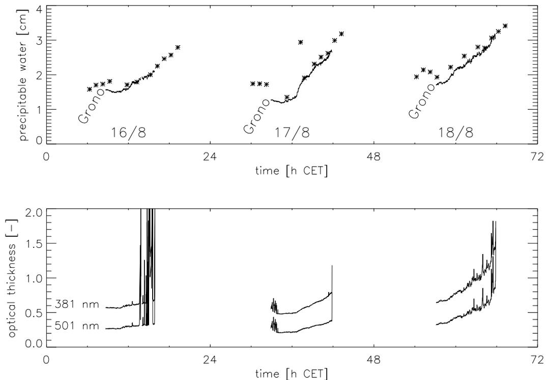
Figure 7 Top: Precipitable water measured by radio sondes (asterisks) and by the solar radiometer (solid line) at Grono. August 16 - 18, 1996. Bottom: Optical thickness of the radiometer channels 1 (381 nm) and 3 (501 nm).
