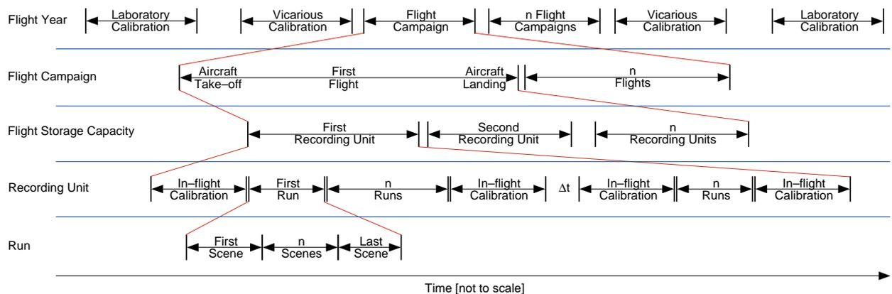
Figure 1. Data Acquisition and Calibration Terminology for APEX
