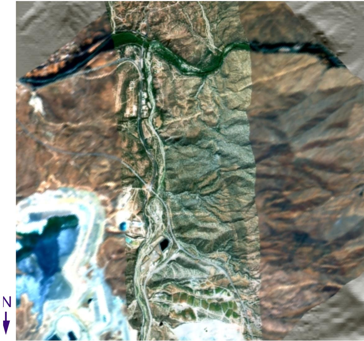
**Figure 1:** Co-registered AVIRIS data over the Ray Mine Area (AZ). Data from a shaded relief, the AVIRIS high altitude scene from June 1998, and the low altitude scene from October 1998 have been overlaid.
