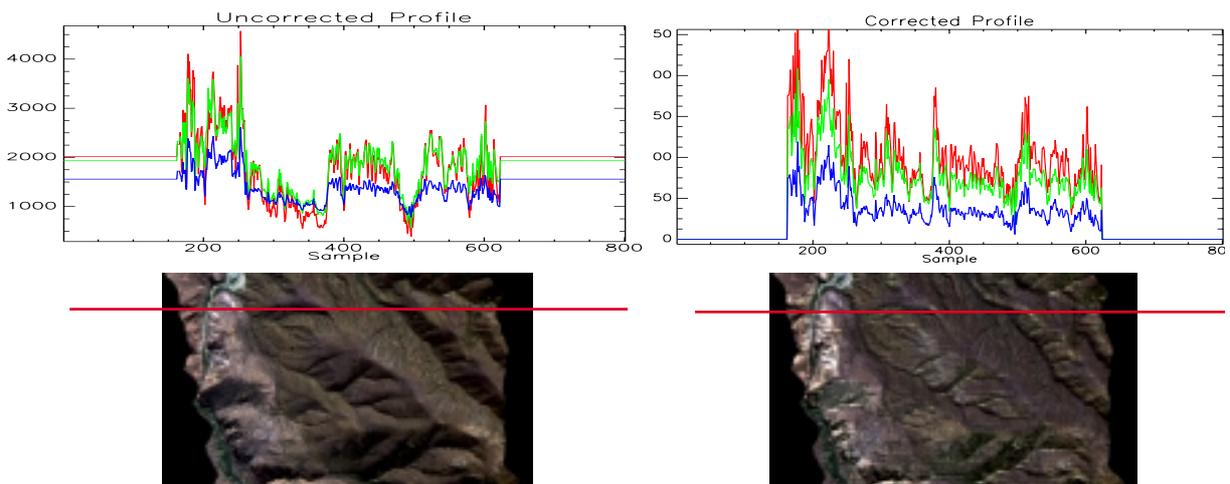
**Figure 4:** Arbitrary profile through the image data, left: uncorrected (scaled at-sensor radiance), right: corrected (surface reflectance).
