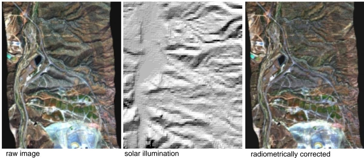
**Figure 3:** Atmospheric/radiometric correction result for the low altitude image data. Terrain shading has almost been eliminated; artefacts still occur due to terrain changes in the mining district, and coarse DEM resolution.
