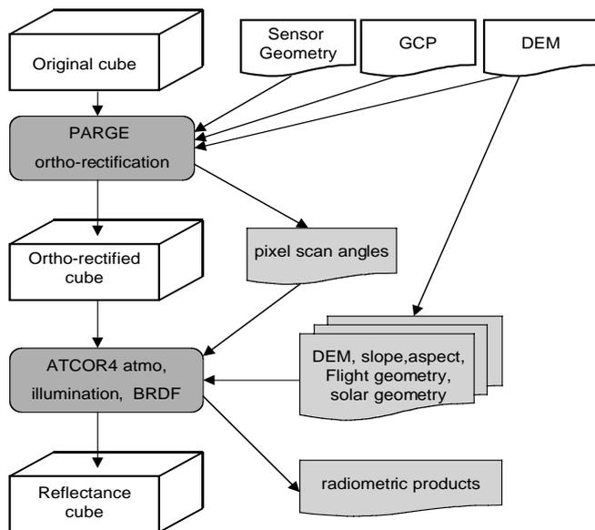
**Figure 2: Process flow of the combined geometric/atmospheric processing chain, including PARGE and ATCOR applications.**
