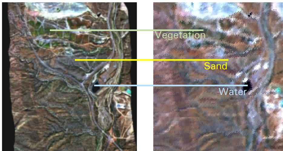
Figure 5: Spectral test areas in the radiometrically corrected and co-registered low altitude data (left) and the high altitude data (right).
