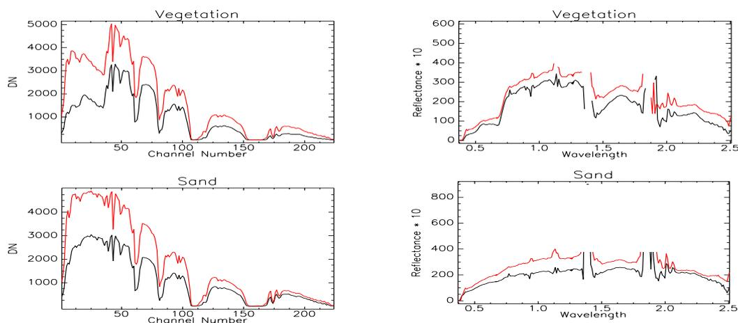
Figure 6: Comparison of multitemporal and -resolution radiometric correction results. Upper curve: 5.6.1998, high altitude, lower curve: 10.3.1998, low altitude.
