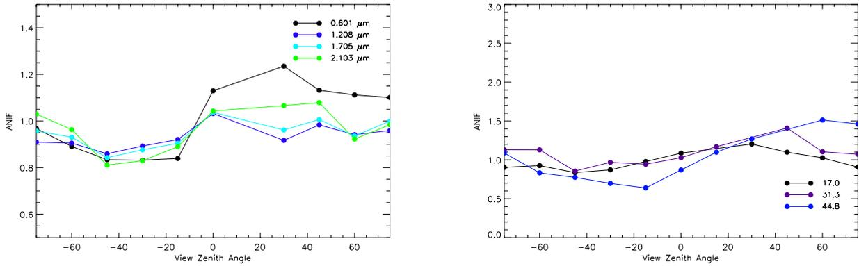
Figure 7: Comparison of normalized reflectances of alfalfa in different wavelength ranges for a sun zenith angle of 22° and a view azimuth angle of 0° (left) and at the wavelength of 0.55 μm for different sun zenith angles (right).
