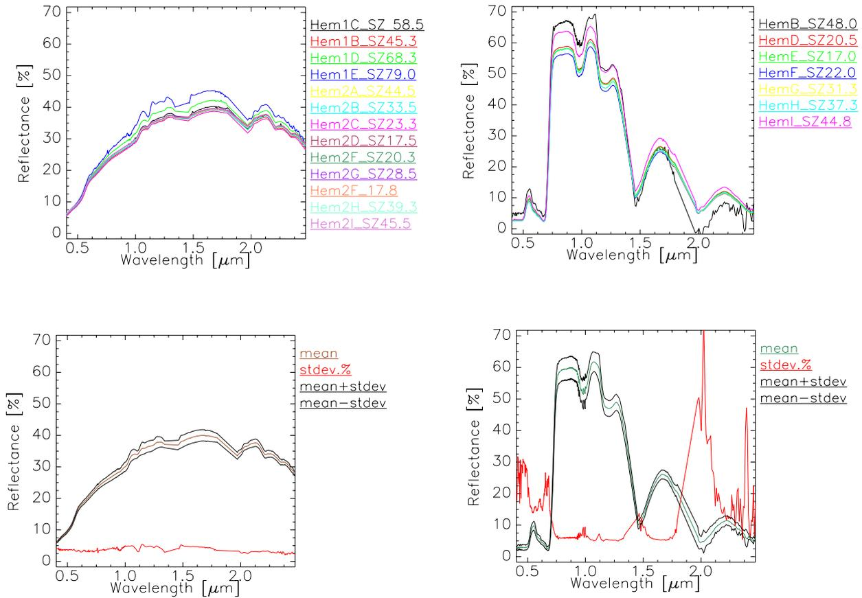
Figure 4: For all hemispheres of bare soil (left) and alfalfa (right) the spectral albedo (top) is computed. Statistical analysis show the standard deviation in percent of the reflectance over the measured wavelength range (bottom).
