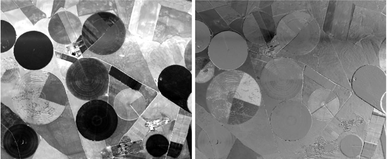
Figure 4: Barrax Co-Registered HyMap data. Left: Raw data at 598 nm wavelength. Right: Difference image between north-south and east-west flight including BRDF effects (Hot Spot) and border effects due to the co-registration errors.
