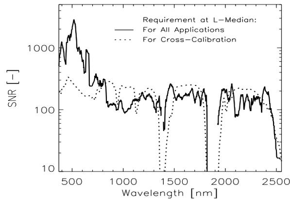
Figure 2 SNR requirements for APEX at median radiance of all applications in comparison to cross-calibration as depicted in Figure 1.
