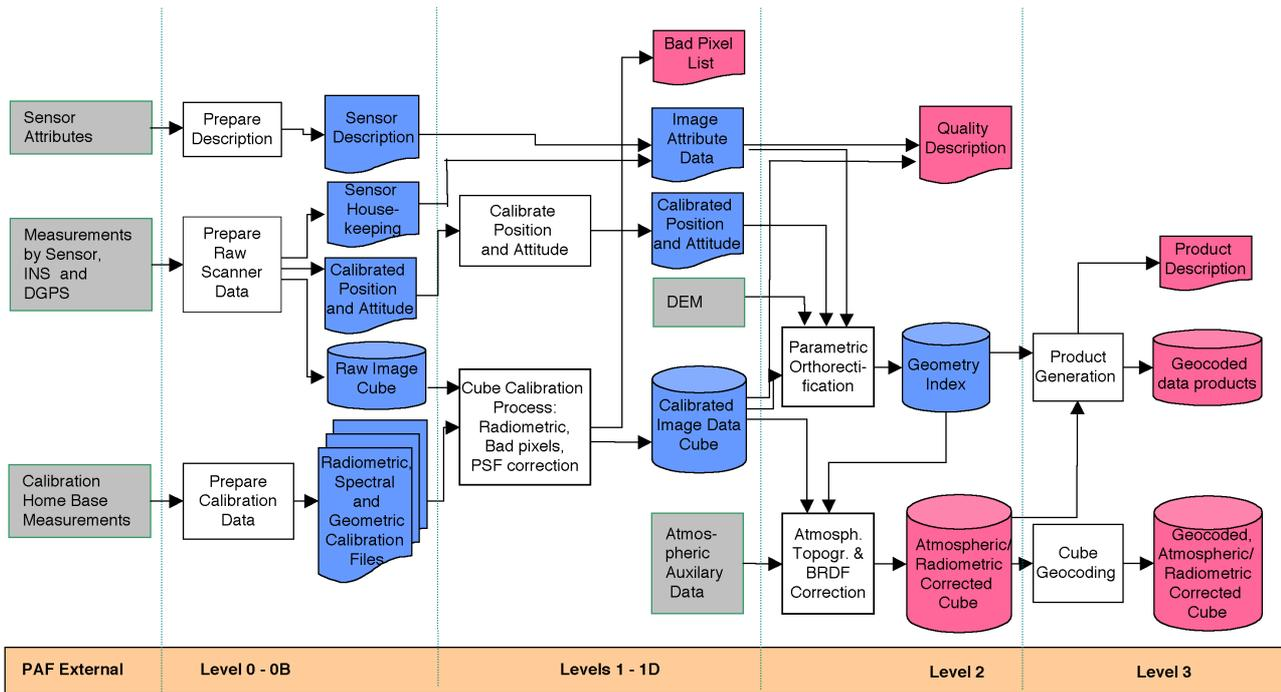
Figure 4 Main data flow for the APEX processing facility
