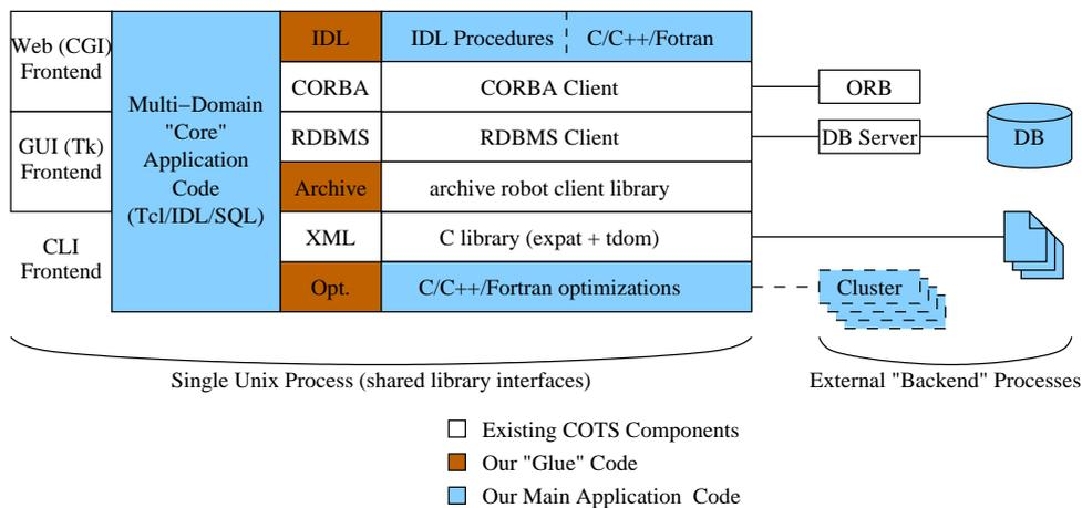
Figure 5 Integrated Processing Engine for the APEX PAF.
