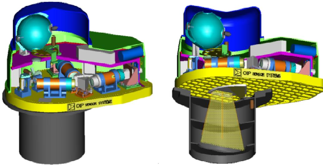
Figure 3 APEX integrated instrument view (left: front; right: bottom-front) (© OIP Sensor Systems 2002)
