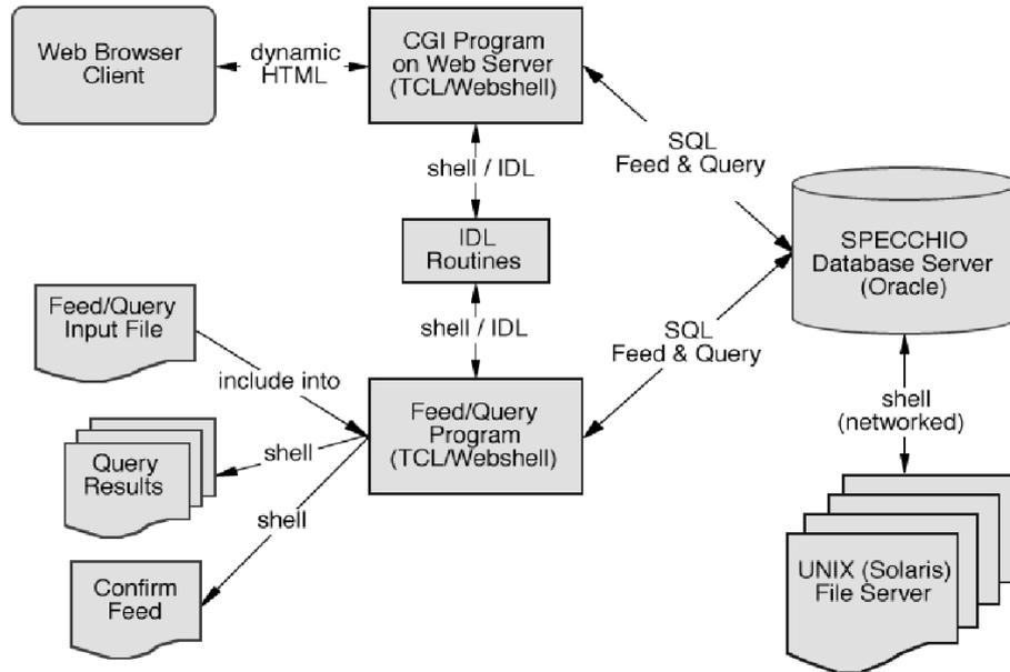
Figure 3: Technical layout of SPECCHIO. Two access interfaces are available: web browser-based (A), or script-based (B). The UNIX file server hosts the spectral source files.
