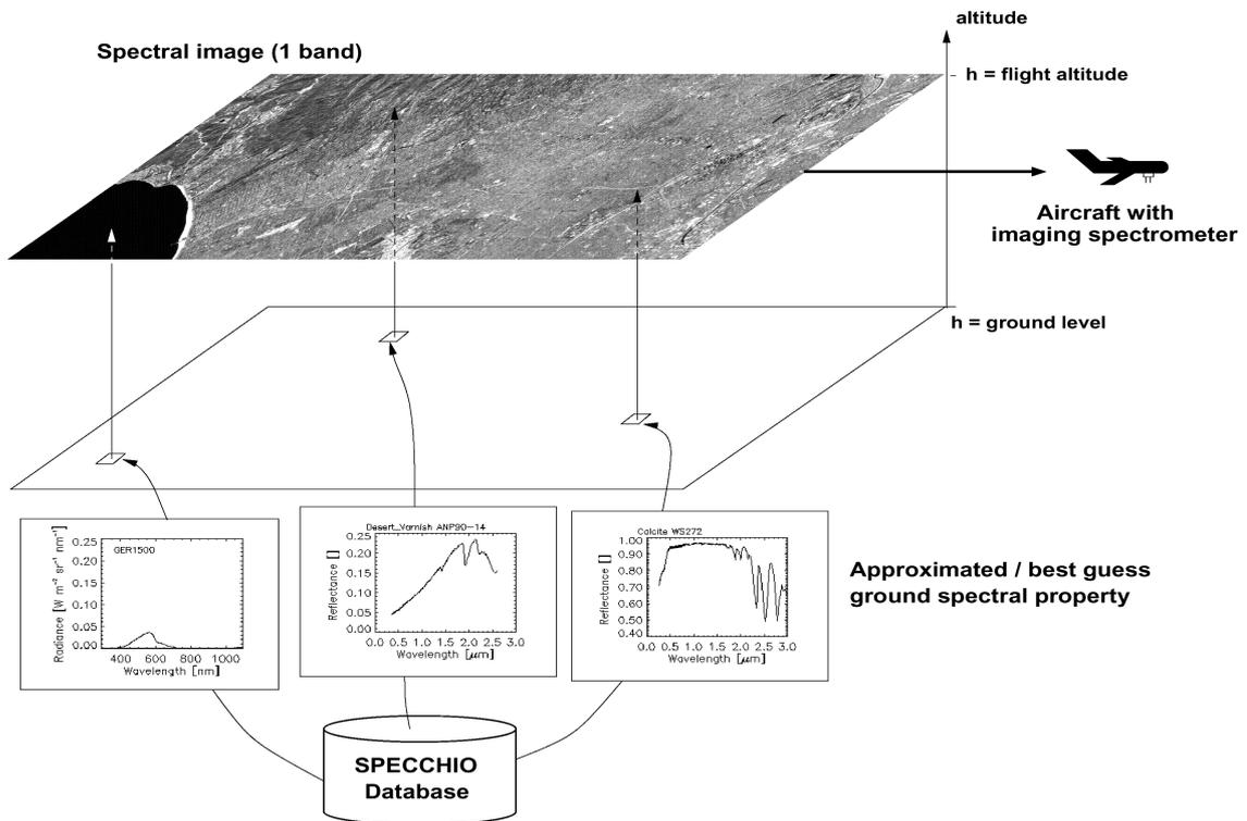
Figure 8: SPECCHIO providing surface spectral information to airborne or spaceborne imaging spectroscopy measurements, aiding in endmember selection for spectral unmixing of the image data.
