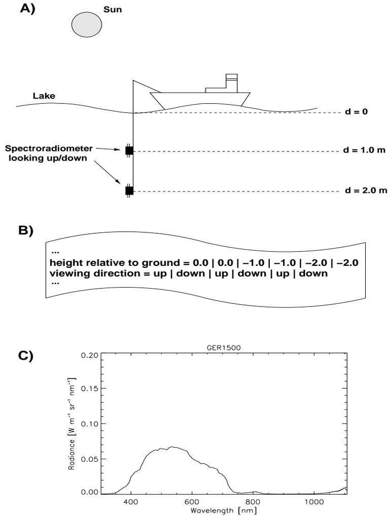
Figure 6: Typical measurement set-up for spectral measurement in lakes in the course of a limnology campaign (A) and part of the corresponding feed text file (B). (C) shows an example plot of downwelling radiance at lake water depth 1.0 m.
