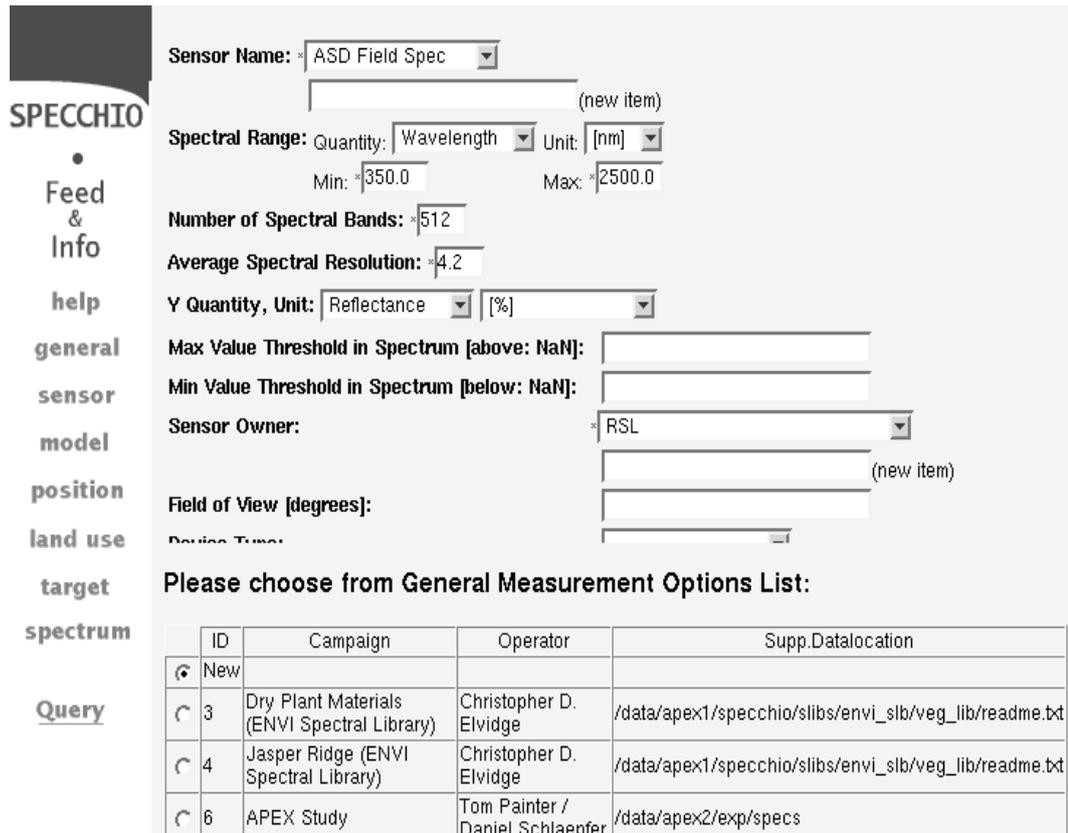
Figure 4: Web interface to feed data into SPECCHIO. The lower main frame of the web site also serves as a view on parts of the current database content.
