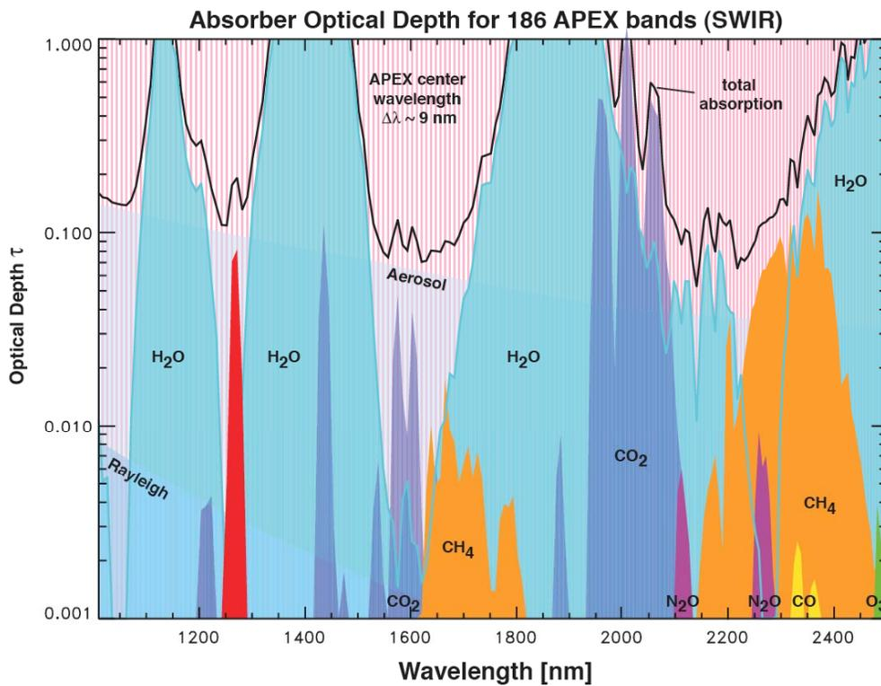
Fig. 2. Atmospheric Constituents' Optical Depths Seen by APEX' SWIR Channel.
