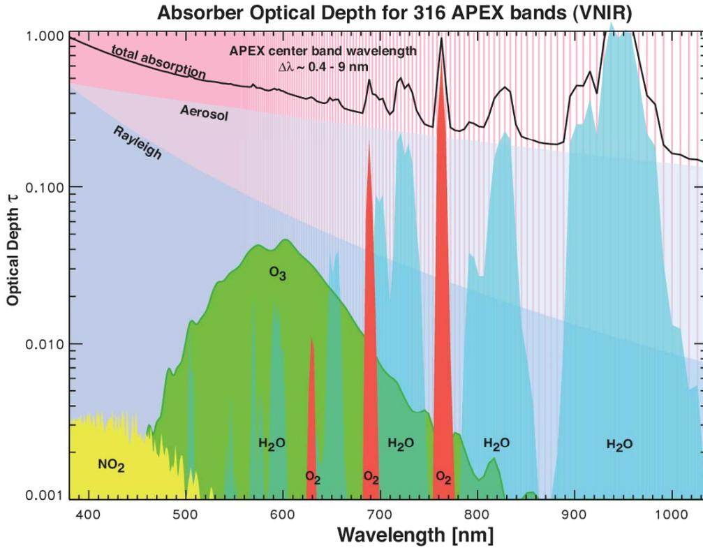
Fig. 1. Atmospheric Constituents' Optical Depths Seen by APEX' VNIR Channel.
